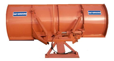
The RB Series plow offers two adjustable coil springs, smooth rolled moldboard, a bottom reinforcement of 5" x 3-1/2" x 5/8" angle and a single 4" diameter reversing cylinder. Single reversing cylinder in conjunction with A-frame allows for closer mounting to truck.
