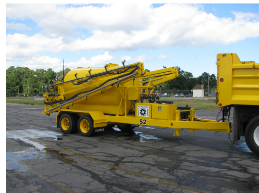
1500 gallon trailer w/75' spray booms Norfolk
