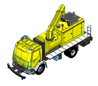
New Rotating Turret - Nozzle and Boom Assembly rotate to stowed position - designed to eliminate operator's obstructed view while equipment is in transport mode
