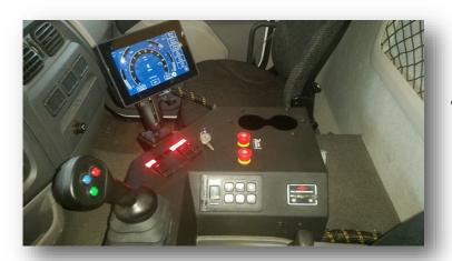
New – 7" Touch Screen display for ease of operation and control - Custom selectable joystick function with proportional control
