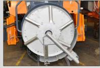
High-speed spreading using Spreading Disc. Efficient spreading at speeds of up to 60
