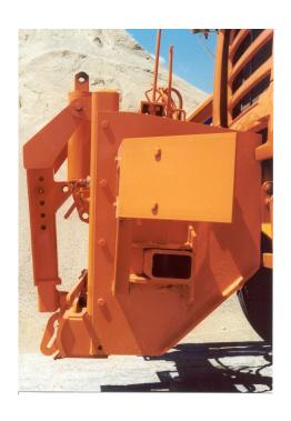
Compact fold down feature for safety and air flow to radiator.
