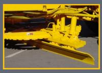
The Poly Patrol Wing has a polyethylene moldboard, full hudraulic lifta dn a trip cutting-edge design. Hydraulic teletube option for maximum visibility throuh passender door window. Left, right and dual mount.
