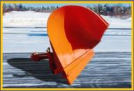
When it comes time to throw and cast snow out of the way, Wausau's HomeSafe One-Way Plow is the answer. Our heavy-duty smooth rolled moldboard with solid welded ribs will stand up to years of hard use. The overhang design is great for driver visibility and eliminating annoying over-spray. Wausau's trip mechanism consists of 3/4" square wire horizontal torsion springs.
