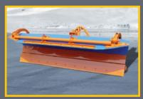
The Reversible AT plow features a spring adjustable trip moldboard to accommodate various edges and road contours.
