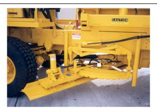
The Underbody Truck Grader is designed so that the operator can apply light, medium, or heavy pressure onto blade depending on task at hand. An accumulator is designed into the plow for safety when hitting and obstruction. Other features include locking cylinders, tilt and hoist, and independent pitch control.
