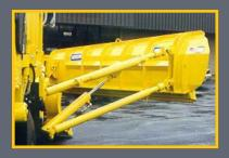
Extending the swath of a front plow, the Space Patrol Wing is designed for benching up to 36". Standard equipment includes an 8" C channel front post, trip moldboard and optional trip edge with parallel.
