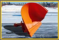
When it comes time to throw and cast snow out of the way, Wausau's HomeSafe One-Way Plow is the answer. Our heavy-duty smooth rolled moldboard with solid welded ribs will stand up to years of hard use. The deep integral shield design is great for driver visibility and eliminating annoying over-spray. Wausau's trip mechanism consists of 3/4" square wire horizontal torsion springs.
