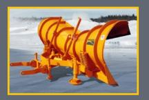
The Expressway Plow is a high speed, reversible trip moldboard snowplow. Dual discharge offers the efficiency of a one-way plow and the versatility of a reversible plow.
