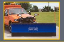
SnoBare is a rugged power reversing trip-edge plow design for medium duty trucks. Standard configuration consists of a poly moldboard, heavy-duty torsion springs and telescopic reversing cylinders.
