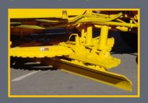
When you need versatility, Wausau's TG Underbody Scraper gives you 3 axes of rotation - reversing, up/down and oscillating side to side for following road contours. The operator can apply light, medium or heavy pressure while the accumulator provides built-in safety when hitting obstructions.
