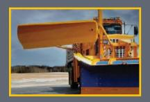
Designed for rugged duty on tandem and 4-wheel drive truck chassis - our high benching wing helps you manage heavy snow accumulation. Flexibility to mount in left, right and dual configurations.
