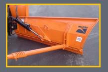
Wausau's Patrol Wing is a full hydraulic lift available with a traditional post or a parallel lift group. Hydraulic teletube option for great visibility through passenger door window. Left, right and dual mount.
