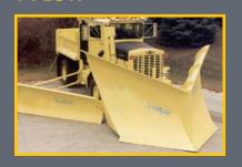
Designed for municipal and highway use when you need to open roads and need high-speed casting and snow removal.
