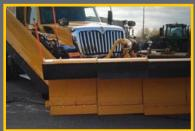
The Street Smart<sup>TM</sup> plow is a multi-section, shock absorbing, reversible snowplow. Each section functions independently to enhance snow removal operation for all types of conditions. Designed for added safety to protect plow, hitch, truck, and operator. Adapts to all types of hitches.
