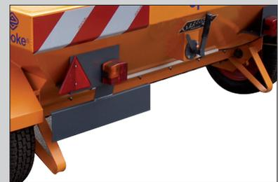
Built-in support feet means simple unloading and towing.
