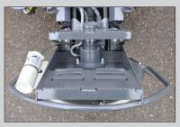
Wide steps on the spreading disc arrangement means safe and easy access to the engine compartment.
