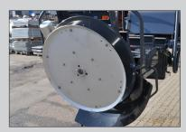
The spreading disc with or without a mixing chamber is selected independently of the spreading material. Efficient spreading at speeds of up to 60 km/h.
