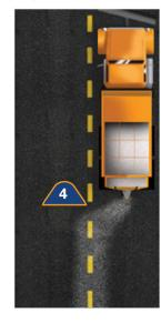
An agitator prevents material bridging and crushes large lumps ensuring accurate material supply. Uniform hopper emptying maintains a consistent center of gravity.
